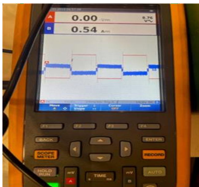
Figure 13: Output of the evolution current using a multimeter in the sediments when pulses are applied.
