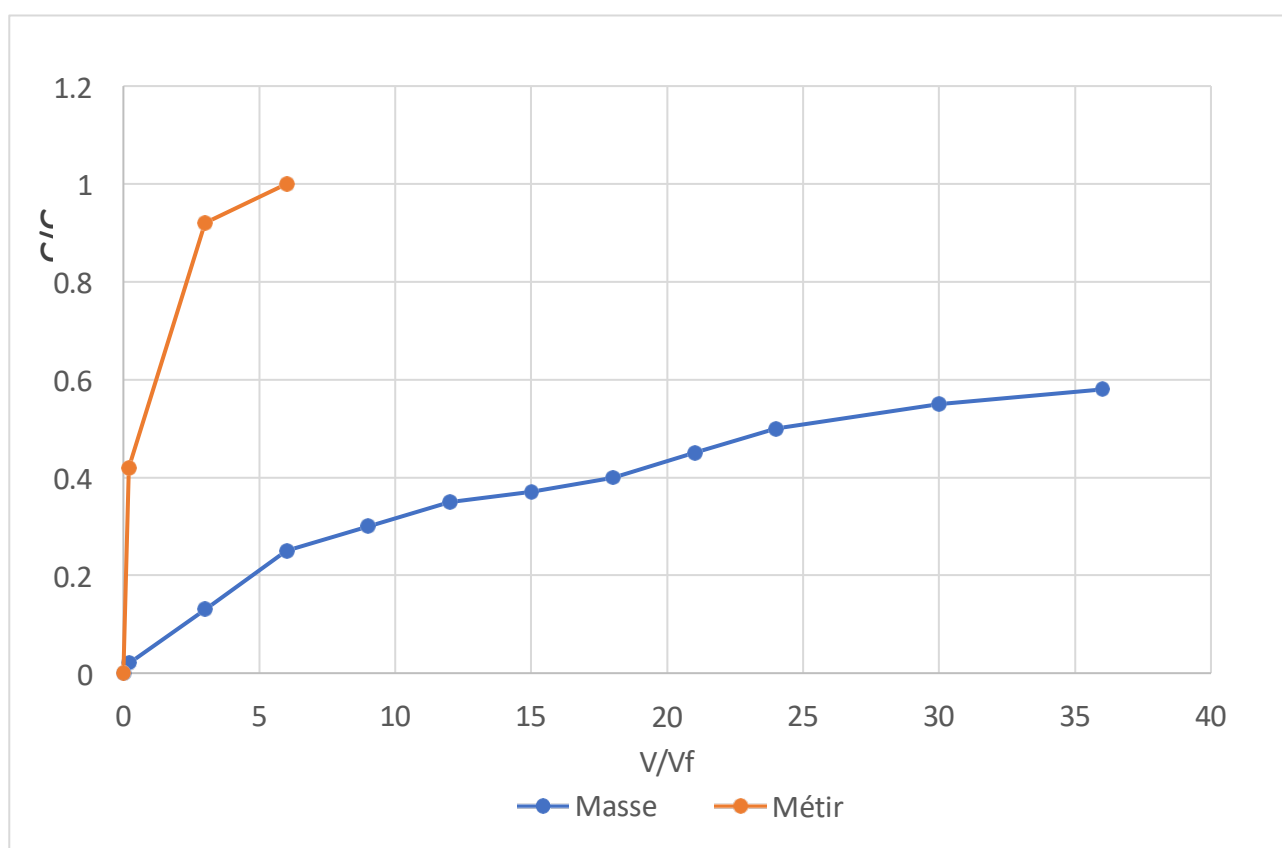
Figure 3: Evolution of the C/C_0 ratio for cadmium for two different supports: "Masse" and "metir".
