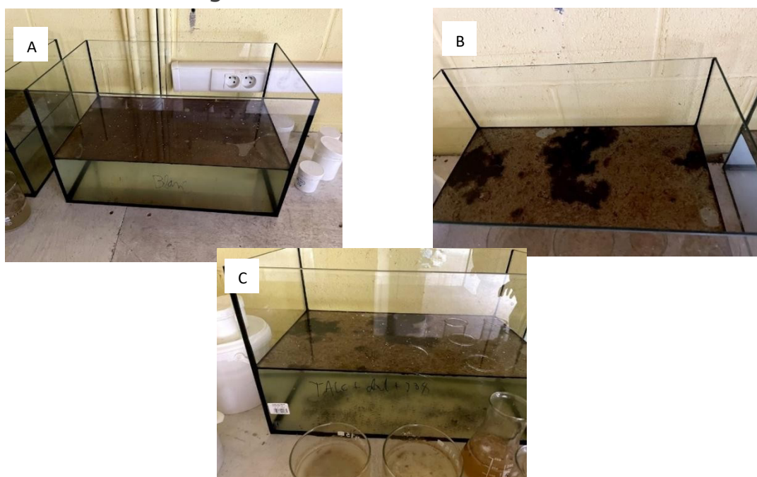
Figure 5: HC capture from support. A) control tank with no supports; B) tank with zeolite; C) tank with a mixture of vulcanic stone and zeolite.
